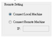
If you want to remote other computer, please choose "Connect Remote Machine", and insert IP. If choose "Connect Remote Machine", you can't send command, scheduling and Shutdown the UPS, but can Shutdown the computer.
