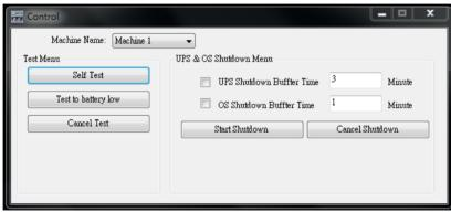
Provides command to UPS for self-test, battery discharge test, stop test, shut-down, stop shut-down and OS for shut-down, stop shut-down.
