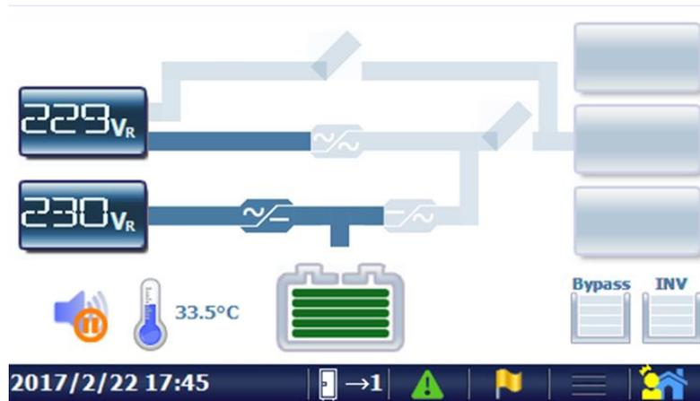
(5) The inverter will be started and supply output voltage.
