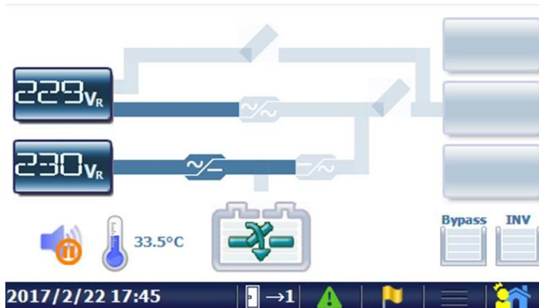
(4) Close the battery line switch/fuses to connect the batteries after rectifier turn on.
