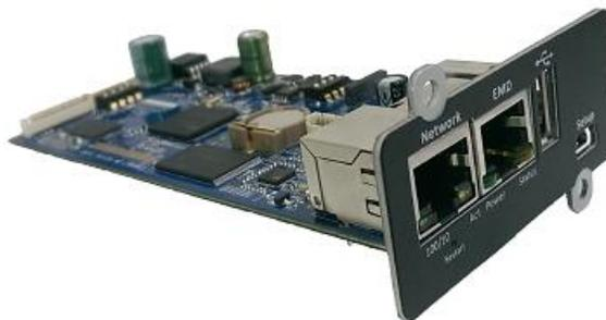
This is the Ethernet network card with TCP/IP, HTTP and SNMP protocols.
