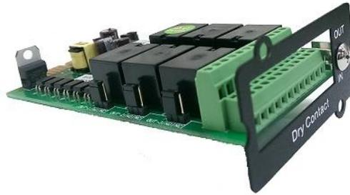
This card provides six output dry contacts and six input contact. These contacts are programmable and user can change the definition for each contact. Please refer to Dry Contact Card manual for more detail.
