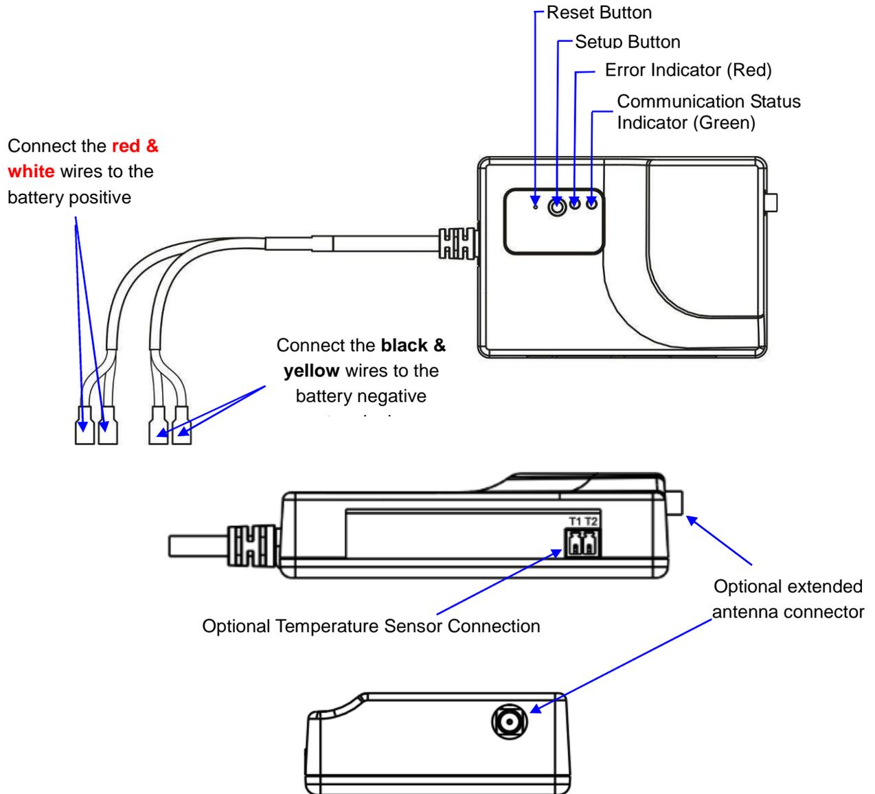
**Figure 4-1. Battery Measure Kit (BMK) External Features**
