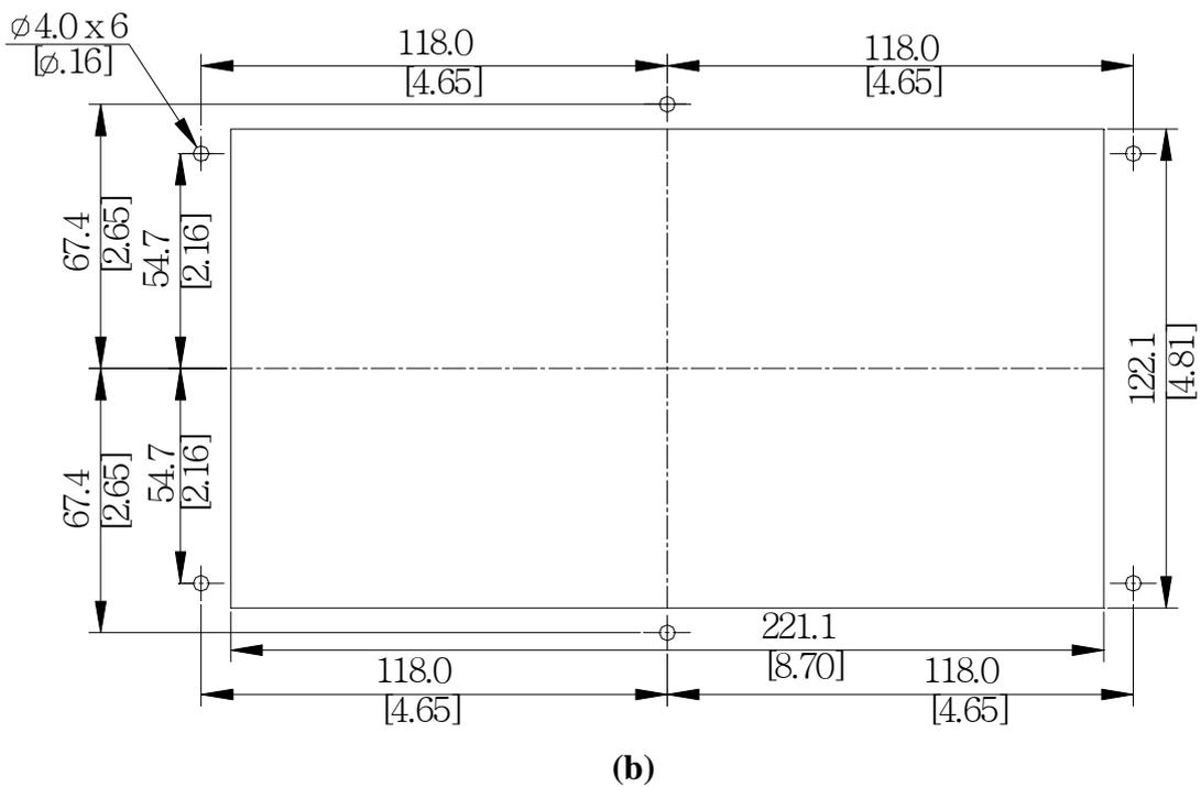
Figure 2-4. Data Collector (DC-LCD II) Fixation Holes
