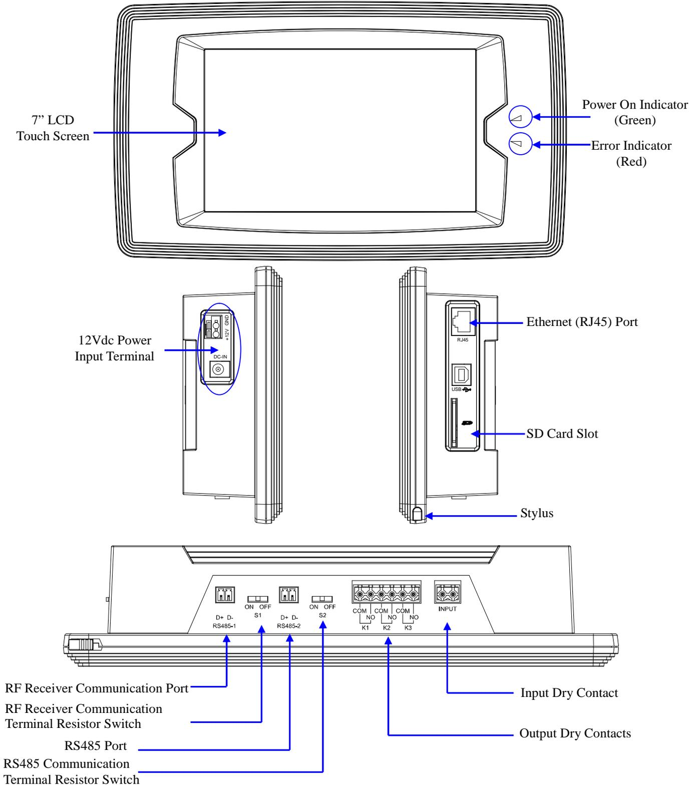
**Figure 2-1. Data Collector (DC-LCD II) External Features**
