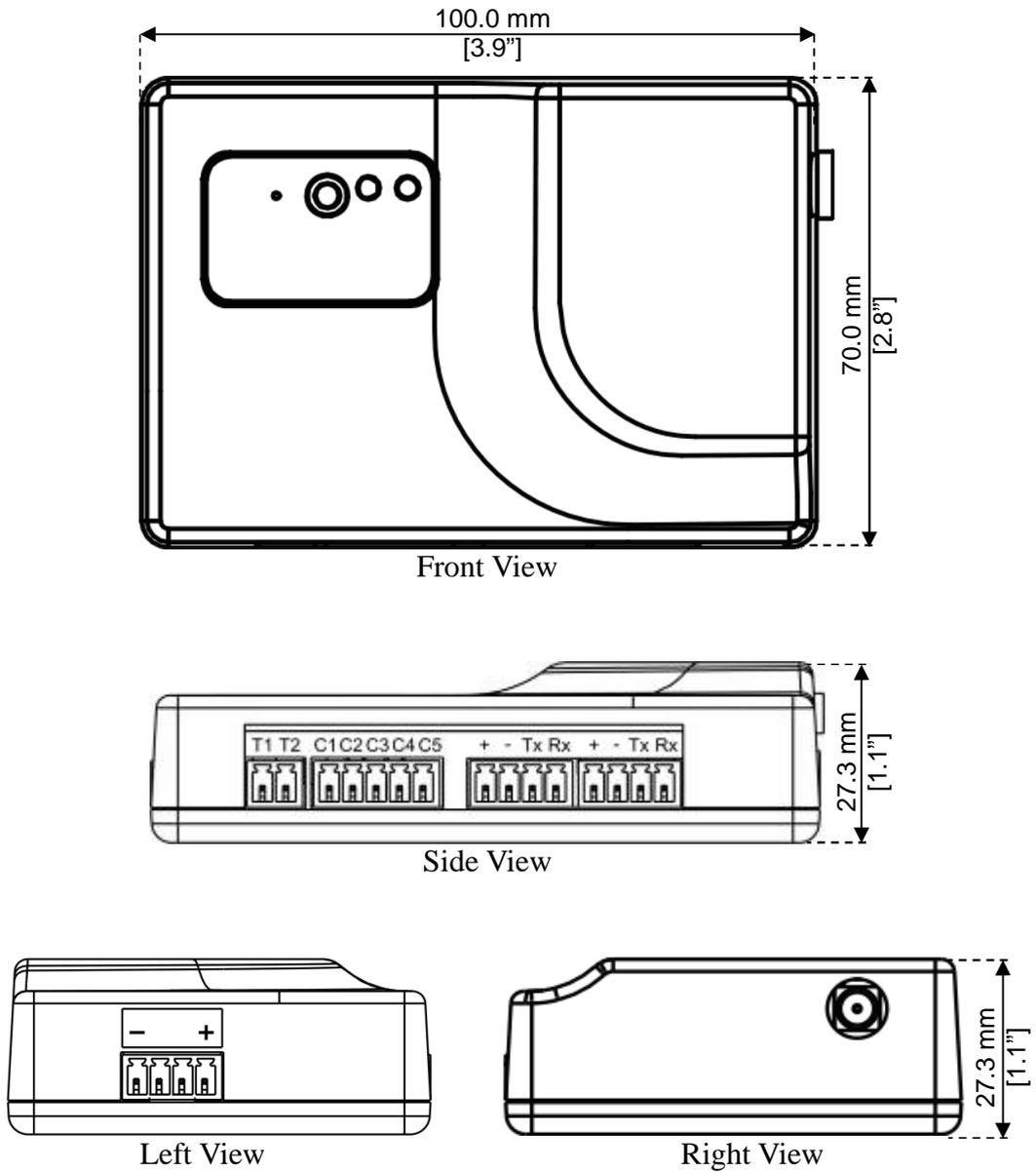
**Figure 5-2. String Measure Kit (SMK) Dimension Drawings**
