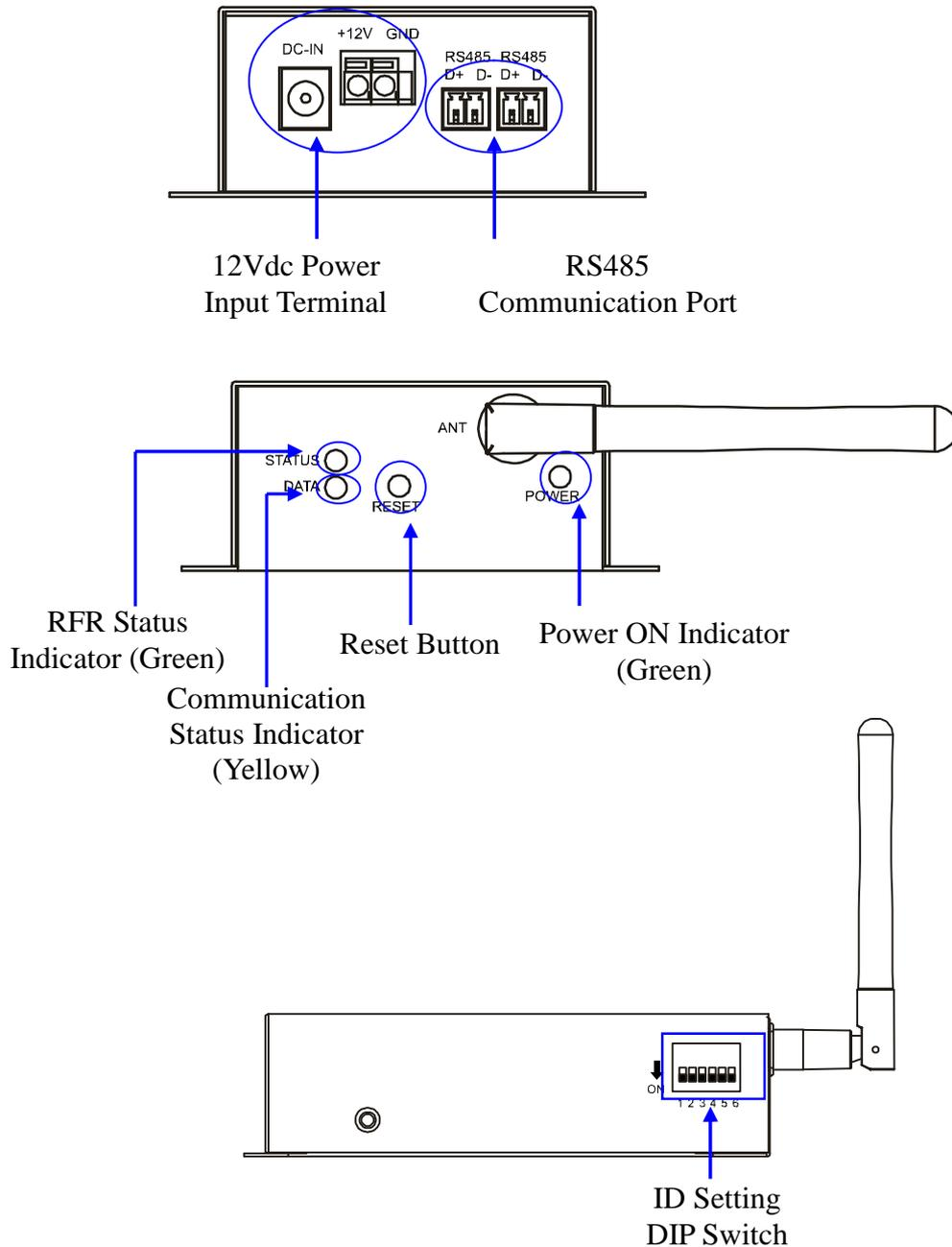
**Figure 3-1. RF Receiver (RFR) External Features**
