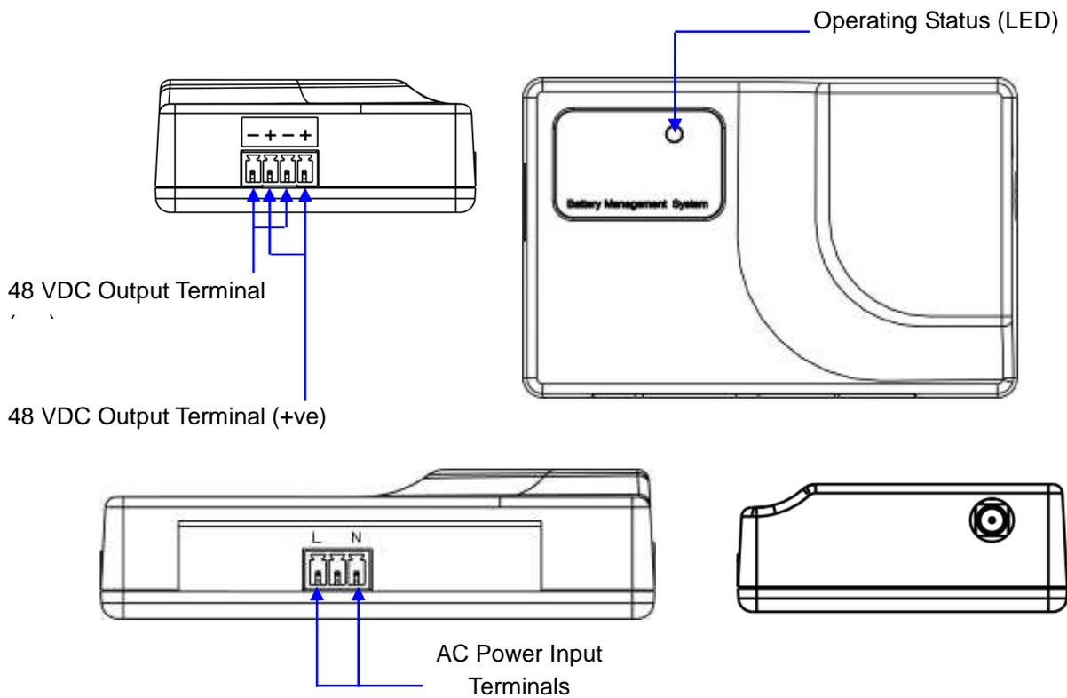
**Figure 6-7. DC Power Supply DPS-048A External Features**
