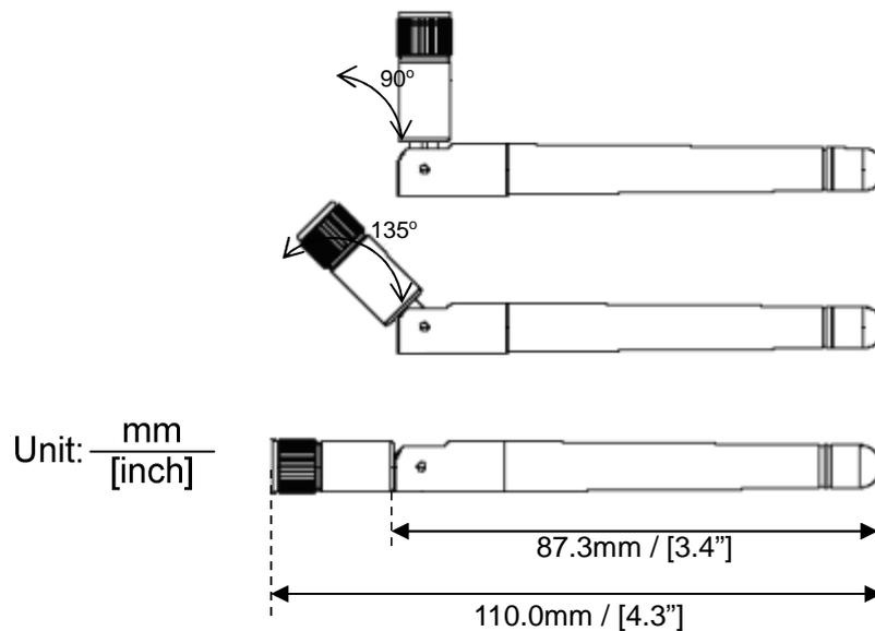
**Figure 6-10. Antenna Dimension Drawing**
