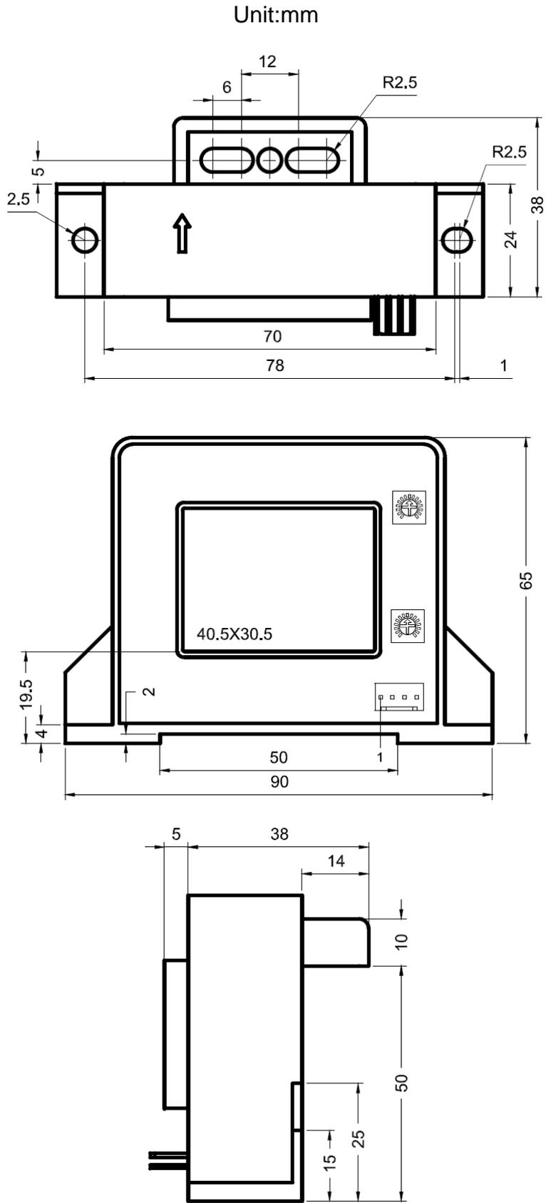
**Figure 6-4. Hall CT Kit (HCT A Type) 200 ~ 1500A Dimension Drawings**
