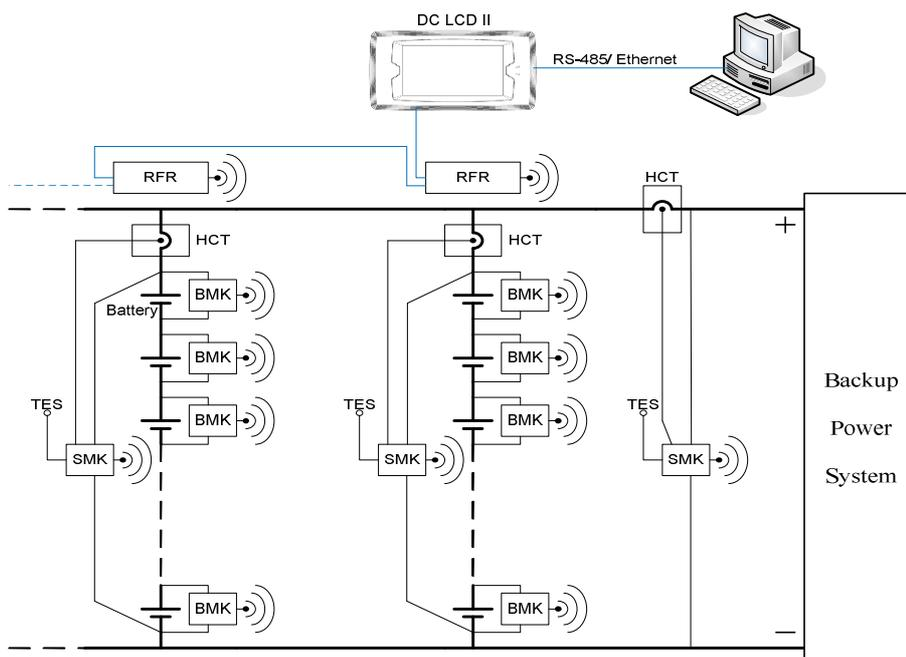
**Figure 1-1. Enerbatt 3G Wireless Battery Monitoring System Configuration**
