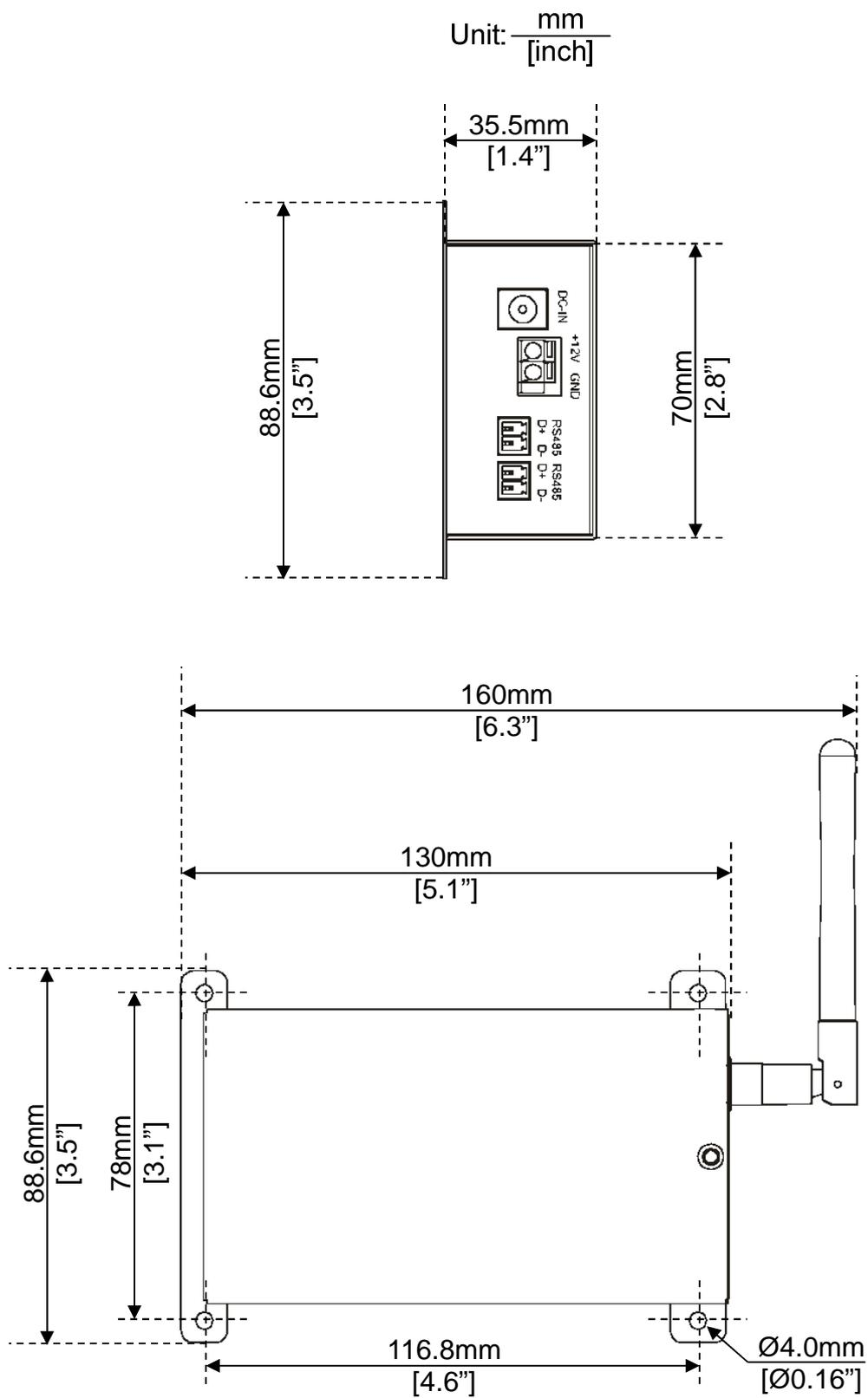
**Figure 3-2. RF Receiver (RFR) Dimension Drawings**
