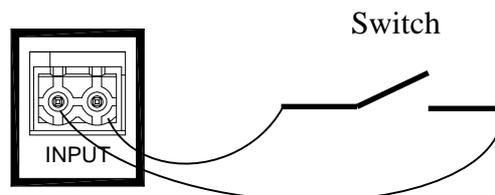
**Figure 2-2. Input Dry Contact Connections**
