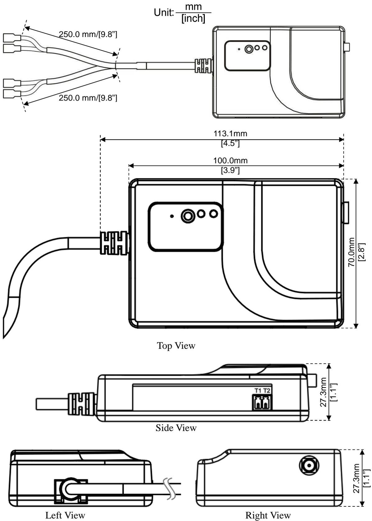
**Figure 4-2. Battery Measure Kit (BMK) Dimension Drawings**
