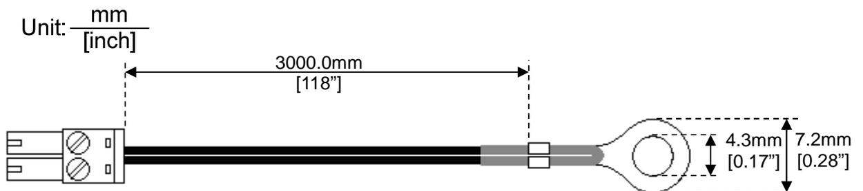
**Figure 6-9. Temperature Sensor (TES) Dimension Drawing**
