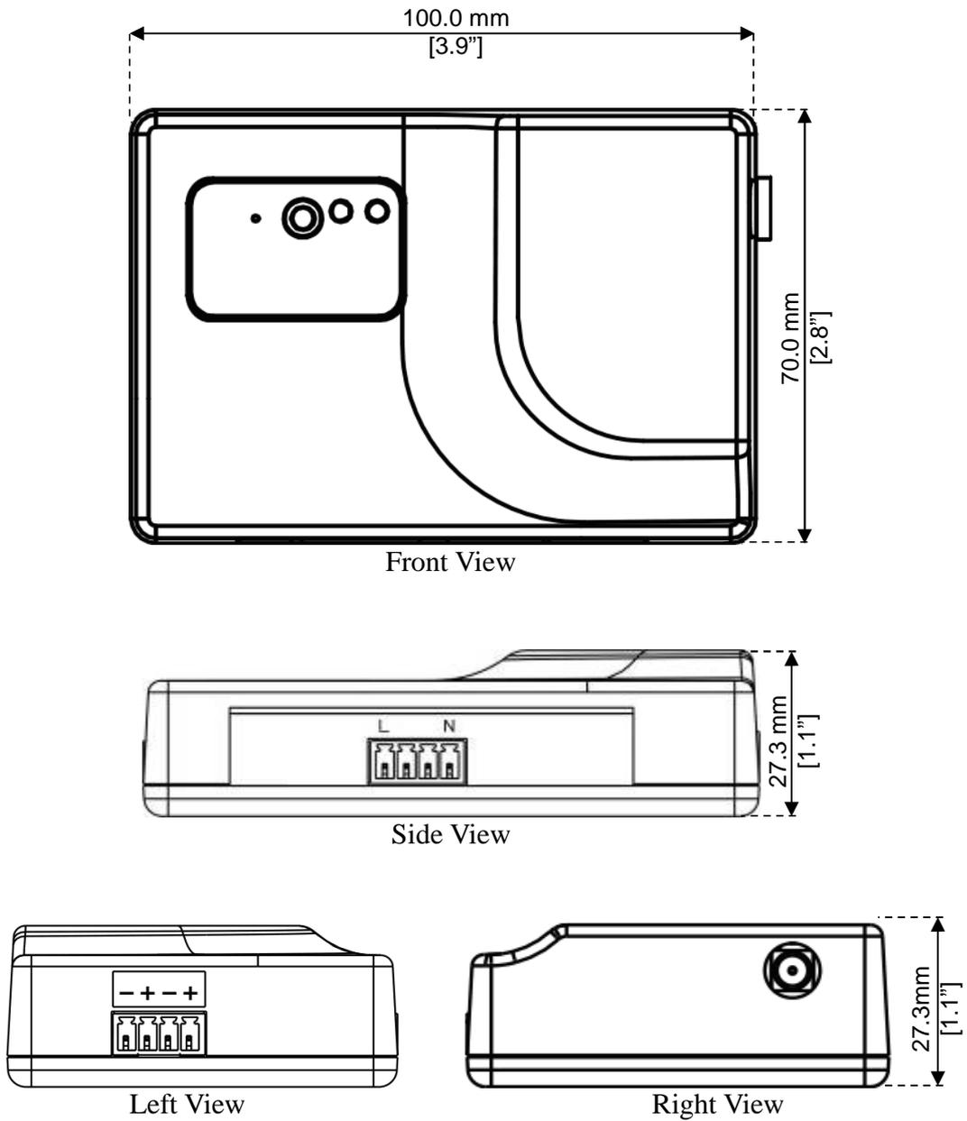
**Figure 6-8. DC Power Supply DPS-048A Dimension Drawings**
